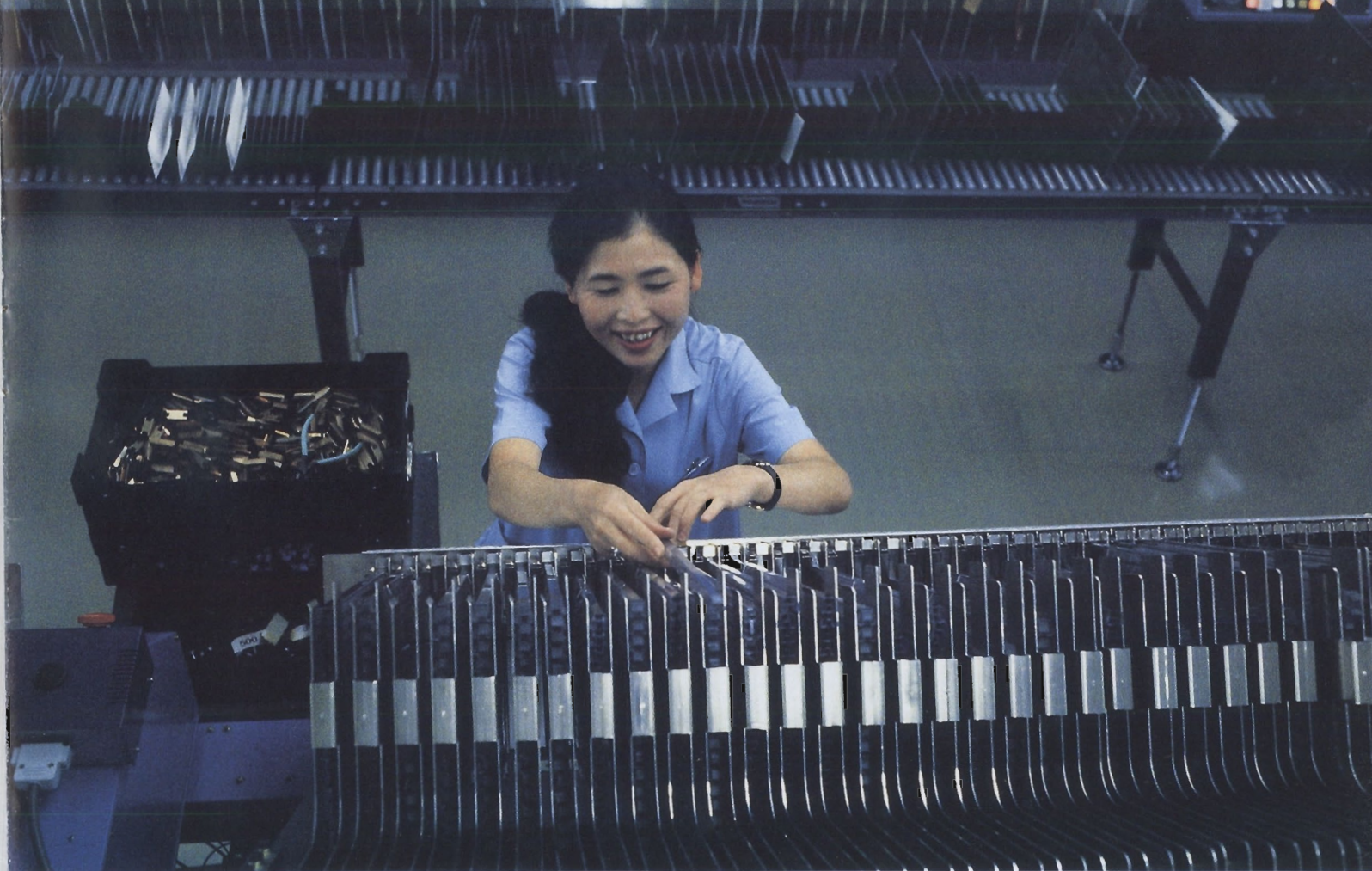
Harumi Aizu sets up integrated-circuit cases on an IC automatic-insertion machine at YHP's manufacturing facility in Hachioji, Japan. Among YHP's considerable successes in the past five years are its 43 percent growth for 1988 and sales topping 128 percent of quota.
